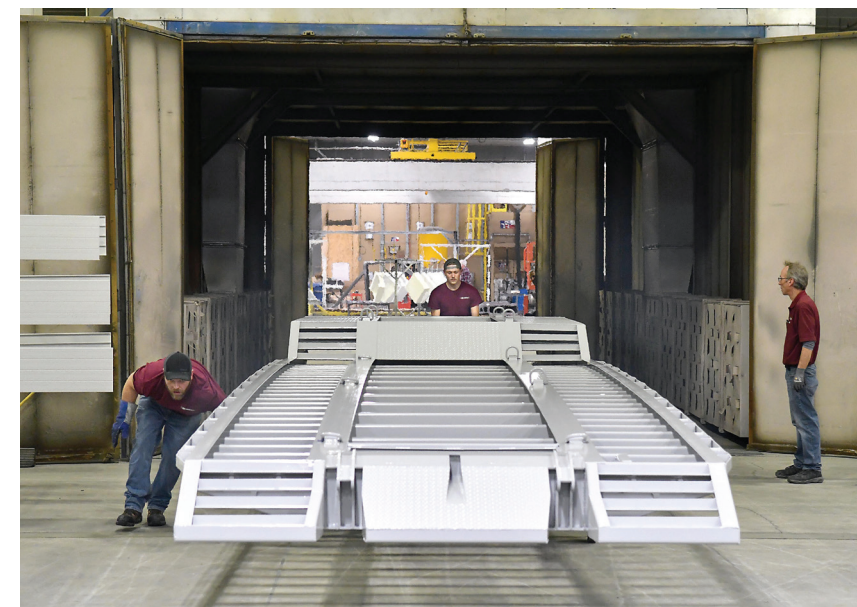
Adam Krueger, left, and Nick Petersen push a powder coated trailer out of an oven at D&K Powder Coating.
